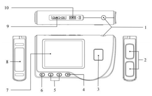
1. **② Power:** Long time press (about 2 seconds) makes the device power on or off; short time press turns on/off the backlight.
